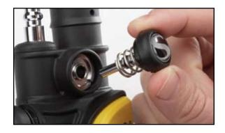
4. Place the poppet seal, o-ring (4) over the threaded end of the Power Inflator Poppet (7). It is not necessary to seat the o-ring in the Poppet. This will occur when the Power Inflator is fully assembled. Assemble the Power Inflator Poppet onto the stem. Finger tight is sufficient.
