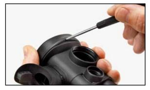
Locate notch in cover and use a small flat blade screwdriver.
