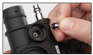
5. Replace the static seal, o-ring (6) on the Power Inflator Valve Cap and thread the cap into the housing. Use needle nose pliers to fasten hand tight.
