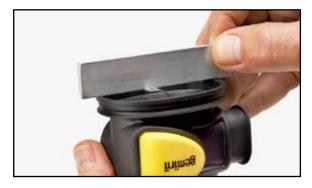
Lever height adjustment even with edge of housing
