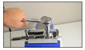
15. Use shop air pressure (less than 125 PSI) applied at the small orifice located in between the spanner slots on the Seat Retainer to dislodge the Seat (16). Discard the Seat.
