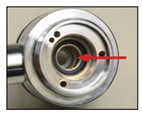
16. Remove Vent Ring (8) and O-ring (7) from the Body. Set aside for cleaning and reassembly.
