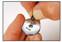
c. Use 20-685-400 Piston Stem O-ring Tool to cover the piston stem threaded end. Slide both the backup rings and the O-ring over the tool to install. The tool will protect the inner sealing surface of the O-ring from being sliced by the piston stem threads. Ensure the correct order of piston guide, backup rings and O-ring. The two back-up rings must have their cupped surfaces against the red O-ring. Picture also shows white piston guide (40) used in SR2 only.
