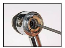
b. Insert the First Stage Seat Retainer Tool into the slots in the Piston Flange to stabilize it while rotating the hex key counterclockwise to separate the Piston Flange from the Piston Stem. This will allow the Spring (5) and the Three-Pin Link (6) to be removed from the Body and set aside for cleaning and reassembly.
