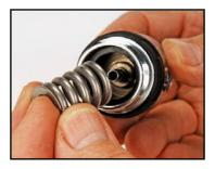
g. Generally lubricate both the Piston Flange exterior O-ring and the sealing surface of the body. While the Piston Stem is secured by the 5/32" hex key go to the other end & start threading the the Piston Flange threaded end clockwise by hand until bottoms, then using the 20-750-150 First Stage Seat Retainer Tool into the slots at the Piston Flange thighten slightly to stabilize it until just snug. Only light torque is sufficient to avoid thread damage.
