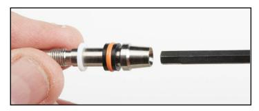
e. Install the Three-Pin Link ensuring that the pins align with the holes in the Body until the Three-Pin Link fully seats inside the Body.
