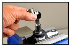
b. Remove the DIN Filter Housing from the Body with a 9/16" open end wrench. Once removed, invert it to allow filter to slide out of the filter Housing.
