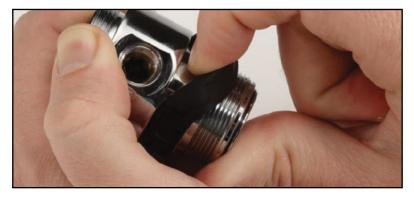
17. Using a soft brass pick or equivalent remove and discard O-ring (15) from the Body at the location where the Seat Retainer was removed. Set aside Body for cleaning and reassembly.
