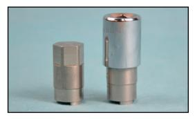
14. Use tool 20-115-100 on one of the HP Ports of the first stage and secure it in the vise. Remove the Seat Retainer (17) by rotating it counterclockwise with the Seat Retainer Tool and socket.
