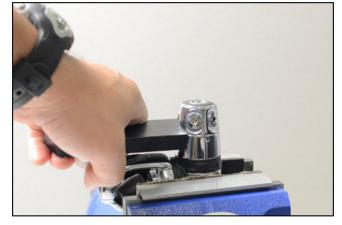
11. Use tool 20-115-100 to stabilize the LP Ports. Place 1/4" hex key in the Swivel Retainer and rotate counterclockwise to separate the End Cap from the Port Swivel. Remove and discard two O-rings (7 and 25). Remove Washer (27) and Accent Ring (23) and set aside for later reassembly.
