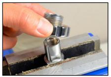
d. Remove and discard O-ring (38). Set aside the Din Handwheel (41), O-rings (35), DIN Inlet Protector (42)
