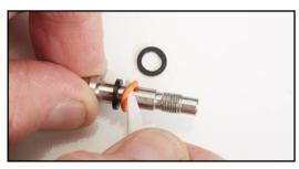
e. It is likely that the Piston Guide (40) will remain inside the body; this one should have to be removed also.
