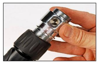
24. Inspect the sealing edge of the Piston Stem using a magnifier. If there are any nicks, cuts or other deformities at the sealing edge the first stage may not provide the high pressure seal needed for the regulator to maintain a stable intermediate pressure. If such damage exists the Piston Stem must be replaced.
