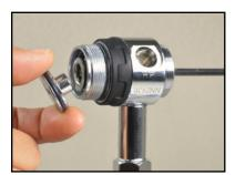
c. Using tool 20-626-400 mount the piston flange to remove inner O-ring as shown. Set aside the piston flange for cleaning, inspection and reassembly.
